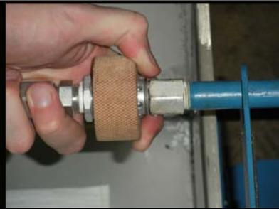
6. Connect discharge hose to pump outlet pipe with snap-tite coupling. Once you securely fasten coupling to pump outlet, twist coupling 180 degrees clockwise.
